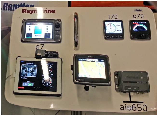
NMEA2000 system with Victron Energy, Raymarine and Empirbus.
